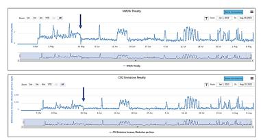
Figure 3. OMNI Condenser performance data showing MW Penalty reduction of 1.05 MW and  $CO_2$  Emissions Penalty reduction of 370 kg/hour after PURATE treatment.
